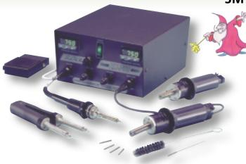
The EX-750 Rework and manufacturing system performs surface mount and conventional component repairs. Tip temperature is electronically controlled from 450 to 900°F (232 to 482°C). Two programmable digital controllers feature responsive closed-loop temperature control with large LED readouts, indicating "Set" and "Operating" temperatures.
