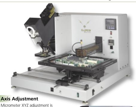
provided on the Board Holder with a motorized Theta axis switch control. Theta in this manner is always "true" and referenced to the component not the PCB.
